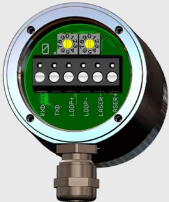
Electrical connections / emissivity adjustment (sensor back side)
