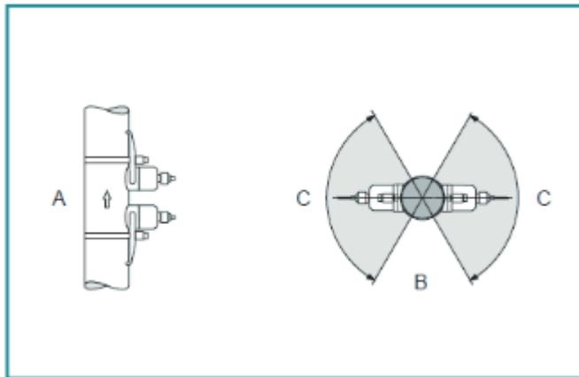
**A** is for upright pipeline, please notice the water direction is from the bottom to top.
