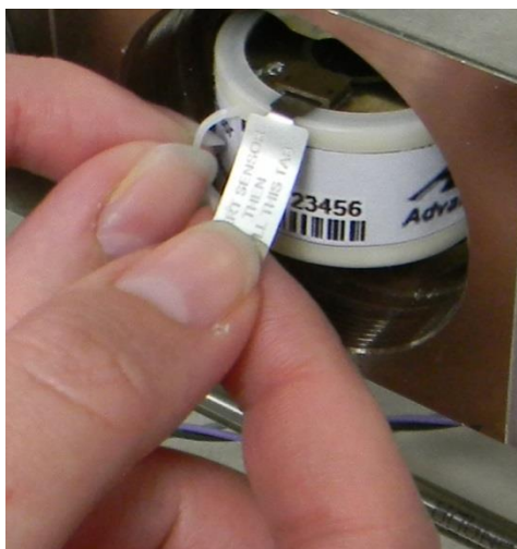
Figure 6. Inserting sensor in cell block
