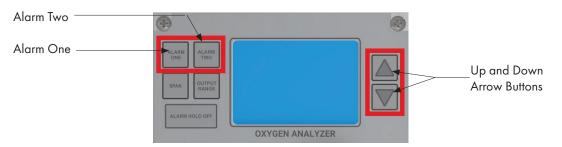
**THE MODEL 2010BX** comes standard with two fully, adjustable independent alarms (ALARM ONE and ALARM TWO).
