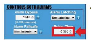
CAUTION: DO NOT adjust this setting unless you are using a pulse-latch slam valve! Otherwise, you will override the relay logic for your Alarms.
