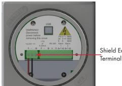
Shield Earth Ground Terminal Connection
