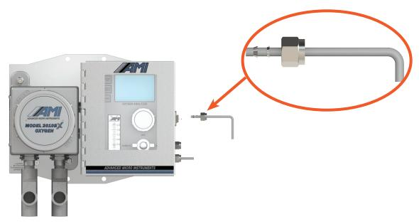
3. Take another deburred length of ¼" stainless steel tubing and slip it through the supplied compression nut and ferrule set. Confirm that the ferrule set is properly oriented and then connect to the EXHAUST PORT.
