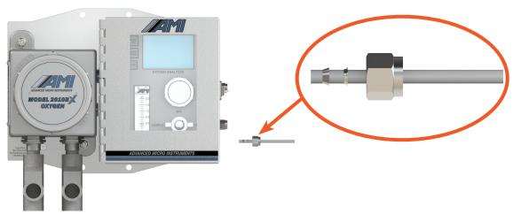
1. Take a deburred length of ¼" stainless steel tubing and slip it through the supplied compression nut and ferrule set. Confirm that the ferrule <u>properly orientated</u> at one end, and connect it to the SAMPLE GAS INLET PORT.
