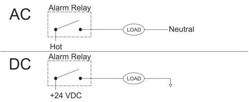
**IMPORTANT**: The relay contacts act like a simple switch breaking only a single leg of the circuit. In keeping with good electrical practices while wiring the alarm contacts, We suggest **SWITCH/BREAK THE HOT LEG only, NOT THE GROUND LEG OF YOUR CIRCUIT**.
