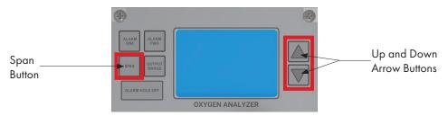
Press the SPAN Button and release. The word SPAN will appear on the LCD for 1 second and then display the oxygen reading, while the PPM FLAG blinks. Quickly press the appropriate UP/DOWN ARROW to adjust the LCD reading to the value stated on your calibration gas cylinder.
