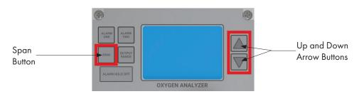
Press the SPAN Button and release. The word SPAN will appear on the LCD for 1 second and then display the oxygen reading, while the % FLAG blinks. Quickly press the appropriate UP/DOWN ARROW to adjust the LCD reading to 20.9%.
