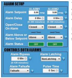
The Analyzer features 2 independent Oxygen Concentration Alarms – one for ALARM 1 and one for ALARM 2. The settings for these alarms, including setpoints, relay contacts, close/open logic and alarm delays, are adjusted through the **COMMAND CENTER**.
