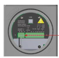
AC Power Ground Terminal Connection (A)
