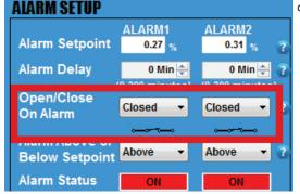
d) Click on the drop-down menu and set the alarm relay contact of each individual ALARM to OPEN or CLOSE when its respective ALARM is triggered.
