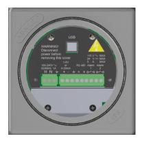
The green terminal block connectors are combination connectors, which allows you to unplug the connector during the wiring process. Combination connectors can accommodate between 12–24 AWG wire for your electrical connection
