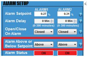
c) Click on the drop-down menu and set the ALARM to trigger ABOVE SETPOINT or BELOW SETPOINT. This causes the alarm flag located on the LCD to illuminate in accordance with your desired setting and the alarm relay contact to open or close as configured in the next step.
