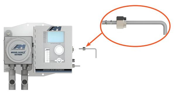
3. Take another deburred length of ¼" stainless steel tubing and slip it through the supplied compression nut and ferrule set. Confirm that the ferrule set is properly oriented and then connect to the EXHAUST PORT.
