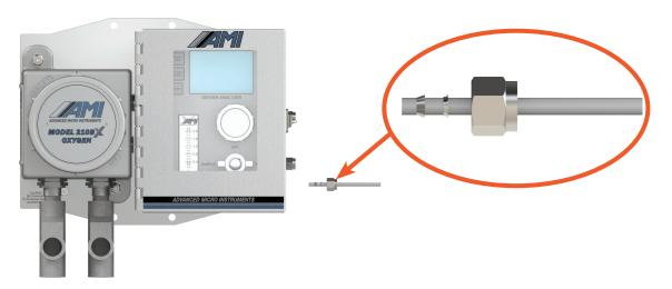
1. Take a deburred length of 1/4" stainless steel tubing and slip it through the supplied compression nut and ferrule set. Confirm that the ferrule <u>properly orientated</u> at one end, and connect it to the SAMPLE GAS INLET PORT.
