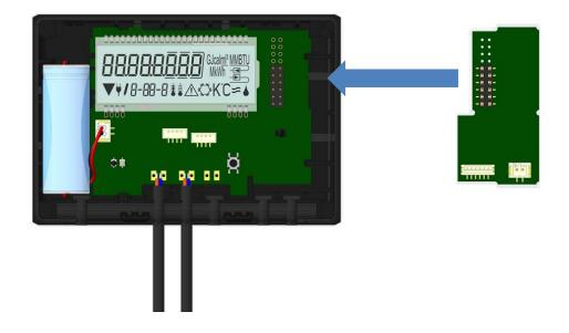
To remove a module the upper housing piece must be carefully pressed against the rear panel of the lower housing piece during opening the calculator. Thus the two rear snap-fits of the upper housing piece lever out the module of the PC board (see picture 4).
