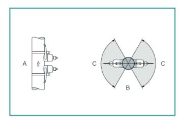
A is for upright pipeline, please notice the water direction is from the bottom to top. B is for horizontal pipeline, the transducers need to be installed inside the C area, angle for area C, max 120°.
